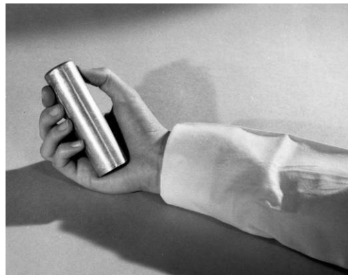
Fig. 4. Graphite Reactor fuel slug.
